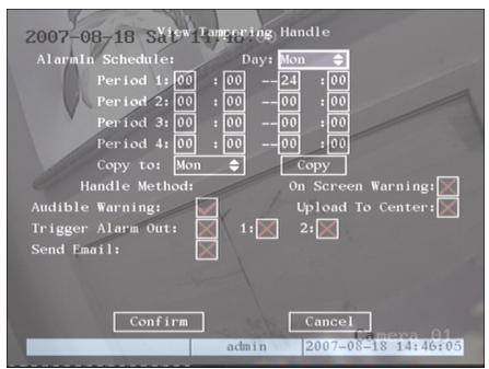
Fig 5.15 View tampering handle setup
